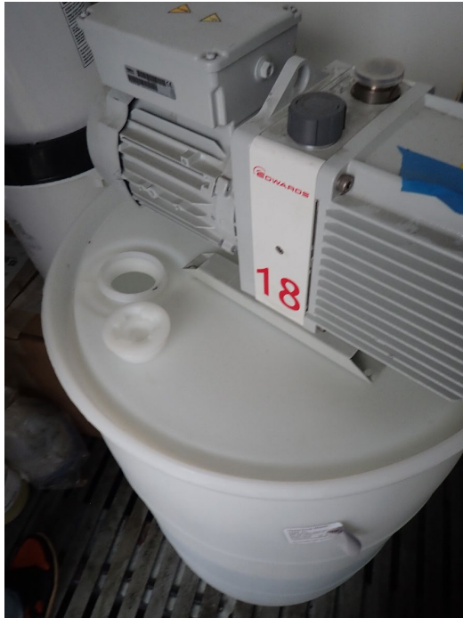
Photograph 5a (P8170020.JPG - 08/17/23): A photo of an open 55-gallon container of “Mega Posit” in Apple’s Bunker Area. At the time of the inspection, the cap was laying on top of the opening of the container (not as depicted here). According to Apple, the container was left opened in order to prevent the container from expanding and bulging.
