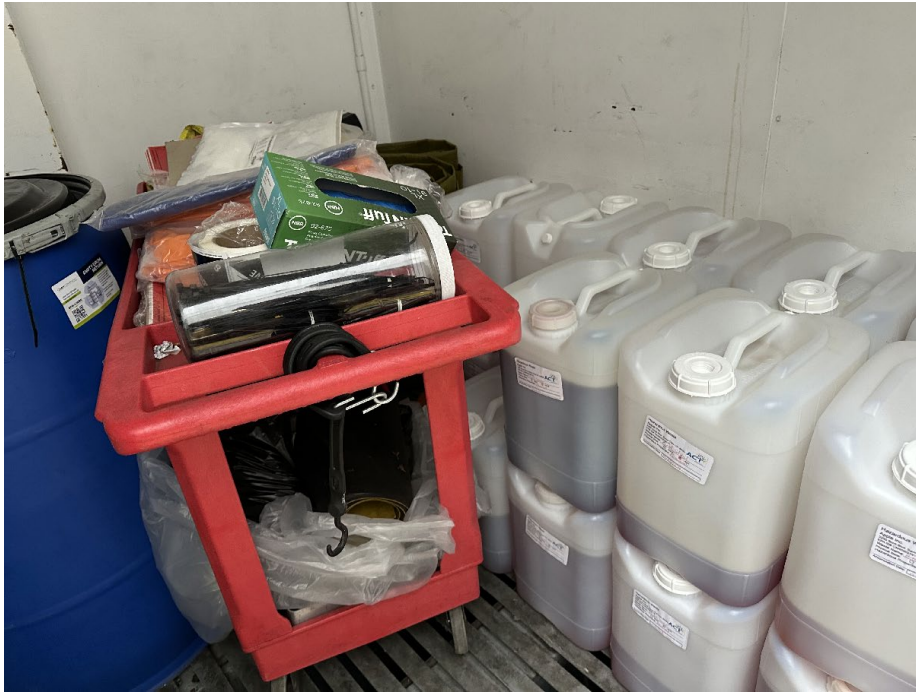
Photograph 13a (IMG_5594.JPG - 01/16/24): A photo of twelve 5-gallon containers of mixed solvent waste in Apple's Bunker Area. The labels on eight of the twelve containers were not clearly visible during the inspection. The waste from these containers were accumulated upstream in Apple's B(4) Area.
