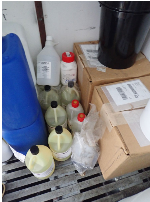
Photograph 4a (P8170016.JPG - 08/17/23): A photo of several containers of expired chemicals on the floor of Apple’s Bunker Area. According to the facility representative, the containers were placed in the Bunker Area that morning and hadn’t been properly labeled with a hazardous waste label or dated, prior to EPA’s arrival.
