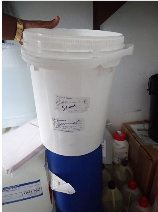
Photograph 3a (P8170015.JPG - 08/17/23): A photo of a 5-gallon container of “Silicone” waste in Apple’s Bunker Area. The container was closed but had an ASD of 03/16/22, more than 90-days from the date of EPA’s inspection. This waste was regulated as a non-RCRA hazardous waste.
